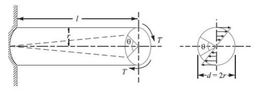
The above equation **is** known as *torsion equation*. It is based on the following a ssumptions:
