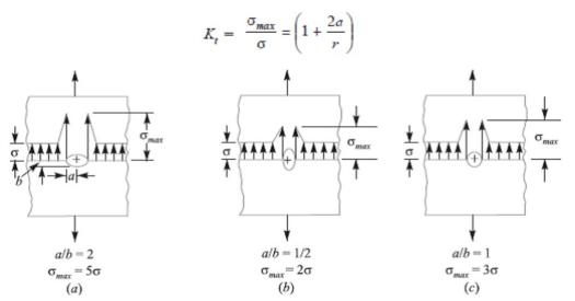
Fig.1. Stress concentration due to holes.
