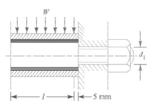
on the pin as shown in Fig. The bush portion of the pin acts as a cantilever beam of length l. Assuming a uniform distributi on of the load W along the bush, the maxi mum bending moment on the pin,
