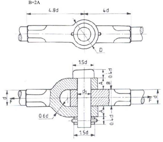
Fig. Knuckle Joint
