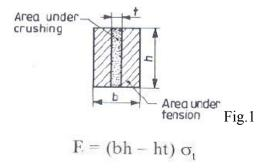
If the rod and strap are made of the same material, and for equality of strength,
