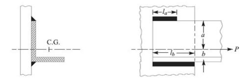
Fig. Axial ly loaded unsymmetrical welded section
