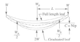
Consider that under maximum load conditions, the stress in all the leaves is equal. Then at maximum load, the total deflection of the graduated leaves will exceed the deflection of the full length leaves by an amount qual to the initial gap *C*. In other words,
