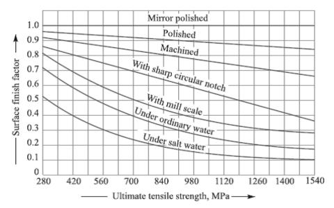
When the surface finish factor is known, then the endurance limit for the material of the machine member may be obtained by multiplying the endurance limit and the surface finish factor. We see that for a mirror polished material, the surface finish factor is unity. In other words, the endurance limit for mirror polished material is maximum and it goes on reducing due to surface condition.
