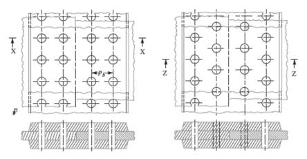
(a) Chain a ri veting. (b) Zig-zag riveting **Fig.** Double riveted double strap (equal) butt joints.
