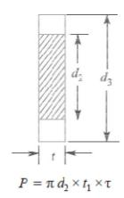
From this equation, the thicknesss of spigot collar (t<sub>1</sub>) may be obtained.
