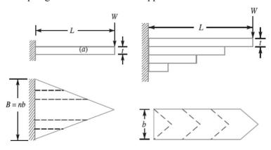
If a triangular plate is used as s hown in Fig., the stress will be uniform throu ghout. If this triangular plate is cut into strips of uniform width and placed one below the other, as shown in Fig. to form a graduated or la minated leaf spring, then
