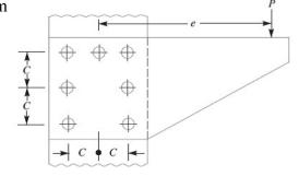
**Solution.** Given: t = 25 mm;  $P = 50 \text{ kN} = 50 \times 103 \text{ N}$ ; e = 400 mm; n = 7; = 65 MPa  $= 65 \text{ N/mm}_2$ ;  $c = 120 \text{ MPa} = 120 \text{ N/mm}^2$ .
