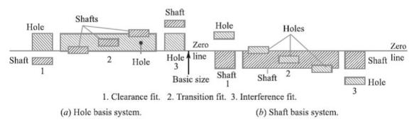
Fig. Bases of Limit System
