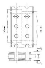
Fig. Single riveted double strap butt joint.
