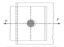
Fig. 7. Crushing of a rivet.
