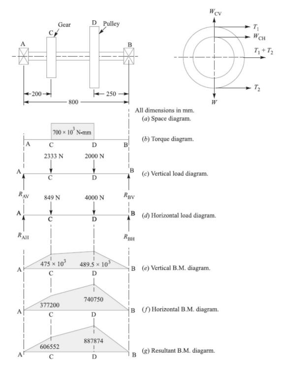
:. Horizontal load acting on the shaft at D,
