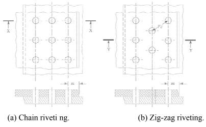
Fig. 9.7. Triple riveted lap joint.
