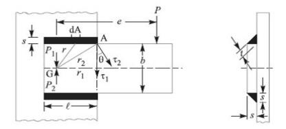
Fig.2 eccentrically loaded welded joint.
