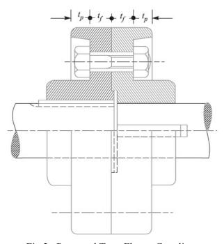
Fig.2 . Protected Type Flange Coupling.
