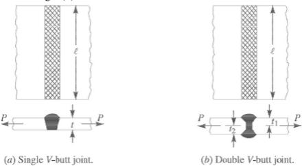
Fig.4. Butt Joints
