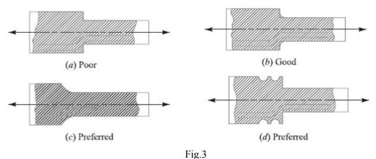
In Fig. 3 (a) we see that stress lin es tend to bunch up and cut very close to the sharp reentrant corner. In order to improve the situation, fillets may be provided, as shown in Fig. 3 (b) and (c) to give more equally spaced flow lines.
