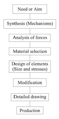
Fig.1. General Machine Design Procedure
