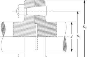
3. <u>Marine type flange coupling</u>. In a marine type flange coupling, the flanges are forged integral with the shafts as shown in Fig.3.
