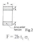
4. Tension failure of the strap across the slot (Fig.3)
