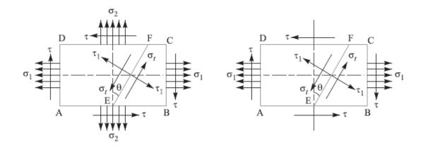
(a) Direct stress in two mutually prependicular planes accompanied prependicular planes accompanied by a simple shear stress.
