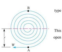
pinned or clamped. Since the radius of curvature of every spiral decreases when the spring is wound up, therefore the material of the spring is in a state of pure bending. Let W = Force applied at the outer end A of the spring,
