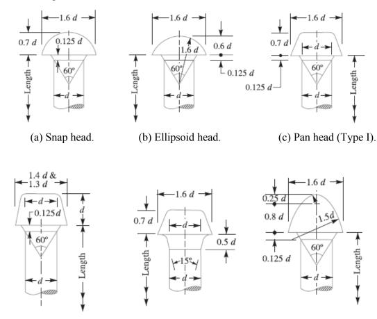
1.4 d for rivets under 24 mm. (e) Pan head with tapered neck. (f) Steeple h ead.
