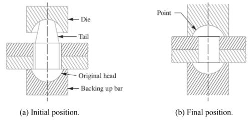
Fig. Methods of riveting.
