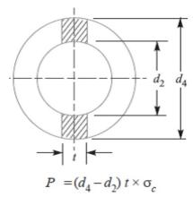
From this equation, the diameter of socket collar (d<sub>4</sub>) may be obtained.
