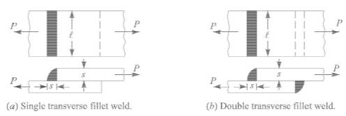
Fig.1 Transverse fillet welds.
