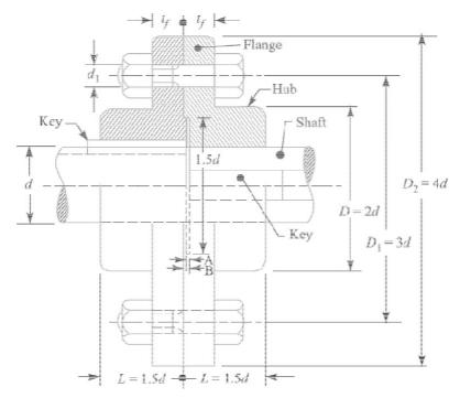
Fig.1 Unprotected Type Flange Coupling.
