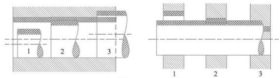
1. Clearance fit. 2. Transition fit. 3. Interference fit.
