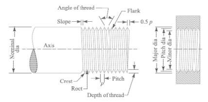
Fig .1 Terms used in screw threads
