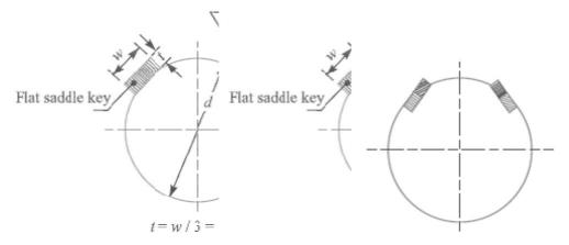
Fig. Flat saddle key and Tangent keys
