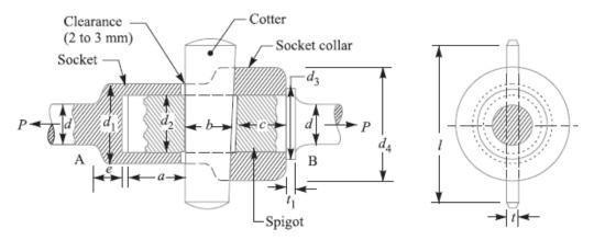
Fig. Socket and spigot cotter joint
