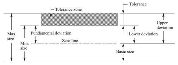
Fig. Fundamental deviation.
