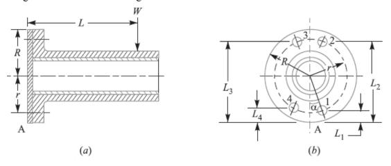
Fig.1. Ecce tric load on a bracket with circular base.
