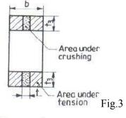
$$F = 2 \ b \ t_3 - 2 \ t \ t_3 = \ 2t_3(b-t) \ \sigma_t$$
