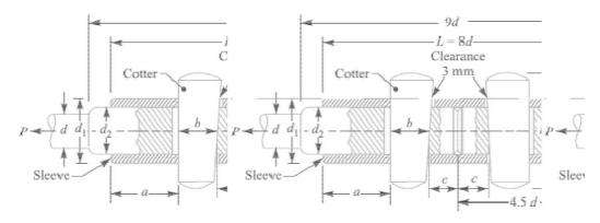
The various proportions for the sleeve and cotter joint in terms of the diameter of rod (d) are as follows:
