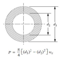
From this equation, the diameter of the spigot collar (d<sub>3</sub>) may be obtained.
