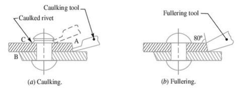
Fig.2. Caulking and fullering.
