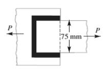
Solution. Given : Width = 75 mm ; Thickness = 12.5 mm ;  $\sigma_{\tau}$  = 70 MPa = 70 N/mm<sup>2</sup> ;  $\tau$  = 56 MPa = 56 N/mm<sup>2</sup>.
