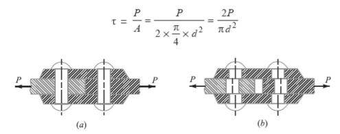
Fig. Double shearing of a riveted joint.
