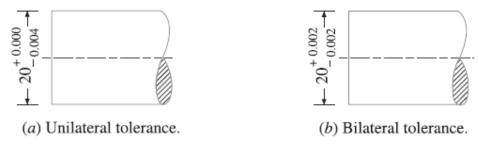
Fig. Method of assigning Tolerances
